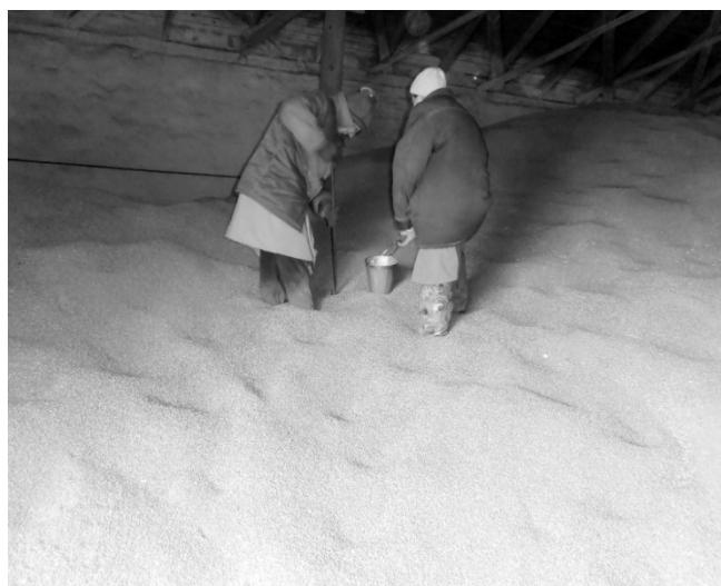
Fig. 2 – The taking of spot samples of grain for analysis of average sample
